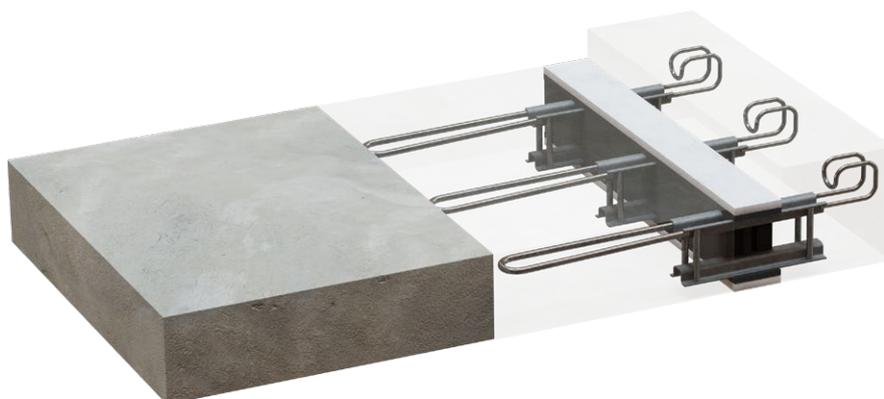
Fig. 12. The TIPOMEGA® connector anchored in the beam using UG4-shaped bars, welded to the upper profile and bent upwards
