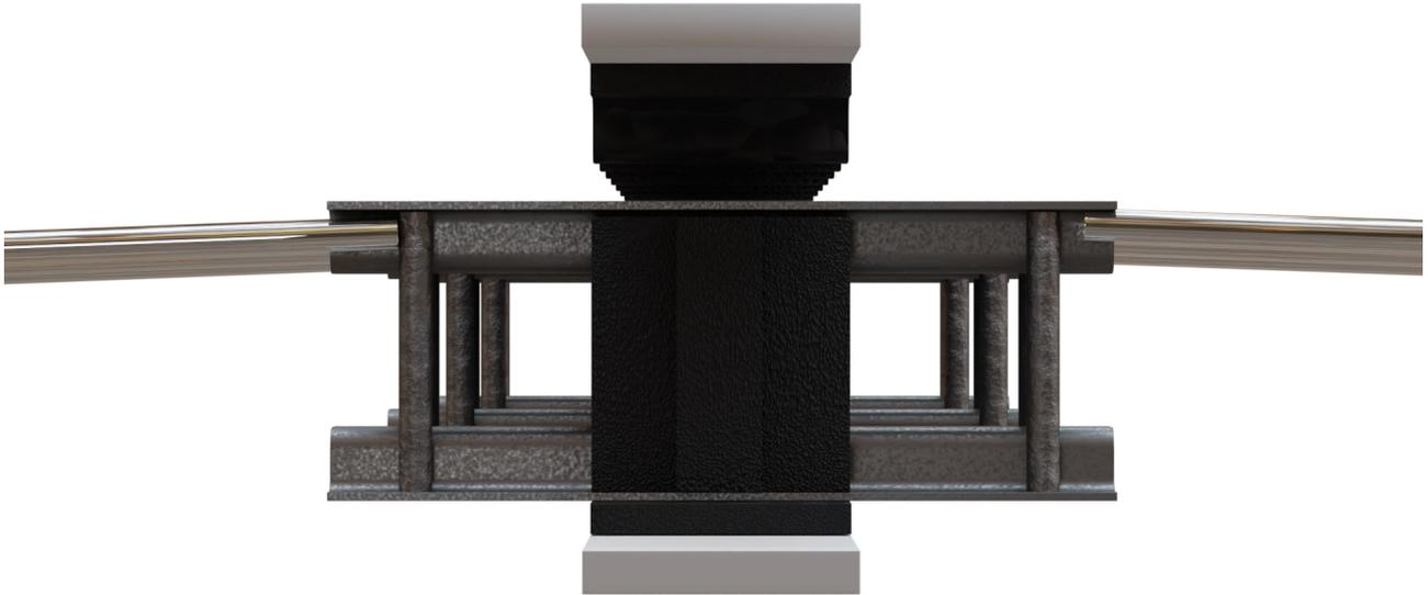
Fig. 35. Symmetrical assembly of the TIP profiles in the OMEGA frames
