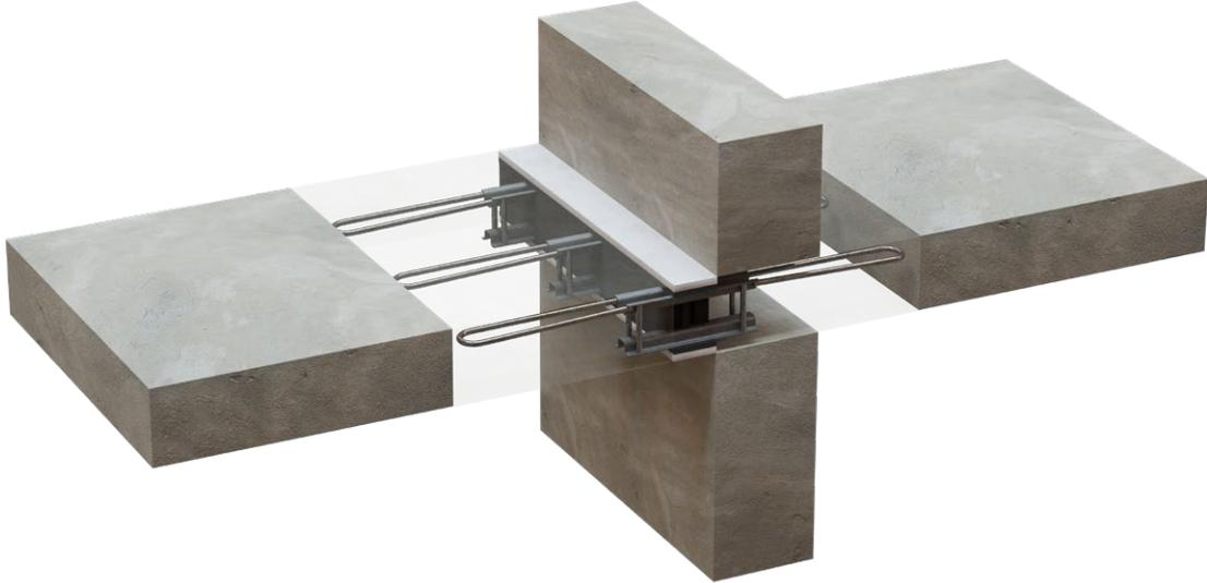
Fig. 3. TIPOMEGA® connector anchored in the floor slab using U1-shaped bars welded to the upper profile
