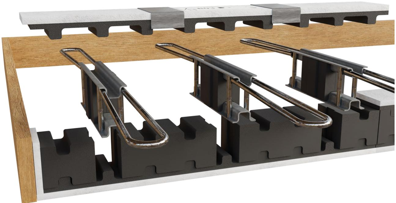
Fig. 36. Assembly of the OMEGA frames in the TIP insulation
