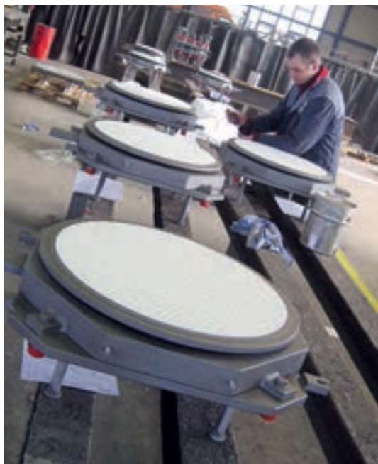
Assembly of free sliding pot bearings
